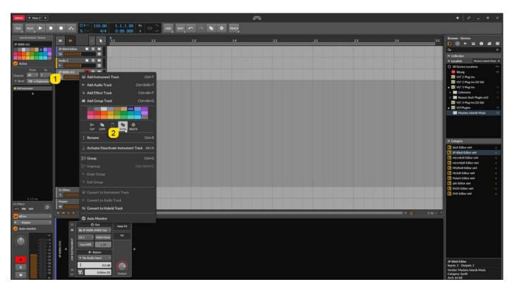
Choose the MIDI out channel [1] to reflect the next part / layer in the hardware and rename [2] the devices to reflect the hardware setup. I will rename my device to "JP-8000 ch2".
