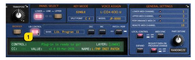
If the LIB CONTROL switch is toggled on and you send a program change message from your master keyboard / controller to the plug-in, it will send the corresponding program from the librarian to the hardware – isn't that just neat?!
