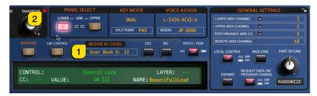
**Note #1** While you have sections locked, there will double the amount of SysEx traffic in the MIDI stream due to the fact that the plug-in has to send the "locked" info back to hardware after the patch is requested. If you scroll patches from librarian, then the data stream is normal.
